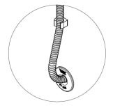
• Shorten flexible protective hose according to requirement and fasten to the wall as required after laying the speed-pipe protection tubes.
