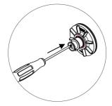
Pierce the rubber seal 3 x 7 mm for the required number of speedpipe protection tubes using a Phillips screwdriver and feed in the speed-pipe protection tubes.
