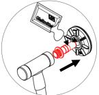
Lubricate the internal sealing element and external clamping sleeve and carefully knock in the sealing element with a soft-faced hammer, until the clamping sleeve flange lies in the intended recess in the sealing element.
