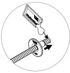
Lubricate flexible protective hose and slide inner cover, support side first, over the protective hose into the hole until the flange lies fully against the wall.
